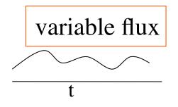
A problem for *synchrotron X-rays*. Solution: Use an external flux meter + scaling.
